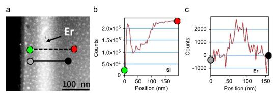
Fig. 4. (a) EFTEM image of Er distribution, (b) EELS Si Profile, and (c) EELS Er Profile.
