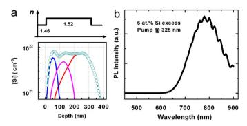
**Fig. 1.** (a) Si concentration and refractive index profiles of the processed waveguides, and (b) the active layer photoluminescence emission.
