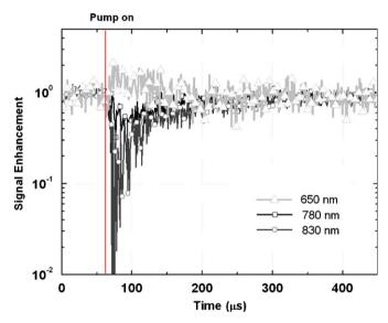
**Fig. 3.** Signal enhancement in log scale for different probe wavelengths. The pump energy density was fixed at 400 mJ/cm<sup>2</sup>.
