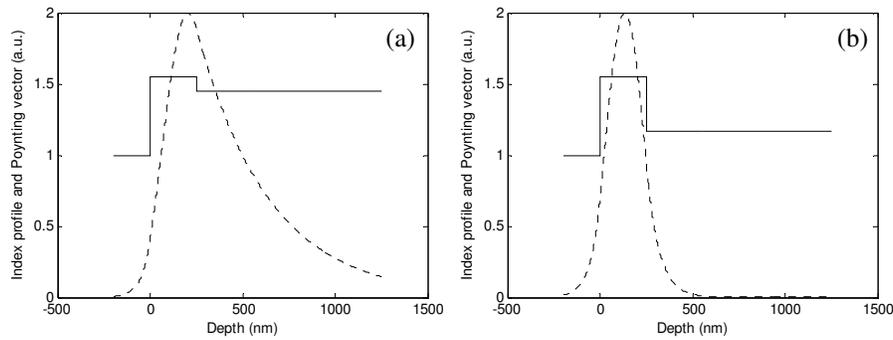
Fig. 5. Mode profiles for a 1.55-index 250nm-thick polymer waveguide with silica cladding with index 1.46 (a) and PS cladding with index 1.18 (b). The confinement factors assuming that all the active layer is excited are respectively 33% and 80%.
