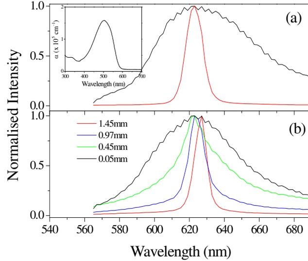
Fig. 2. (a) Normalized emission spectra of sample 3 above and below the ASE threshold. The inset shows the optical absorption coefficient of the MEH-PPV polymer. (b) Normalized emission spectra of sample 3 at a pump power above the ASE threshold as a function of the excitation stripe length.
