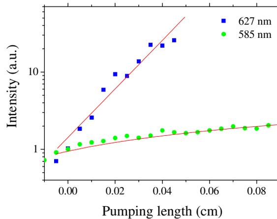
Fig. 3. ASE intensity at 627 nm (blue squares), and at 585 nm (green circles) as a function of the illumination length at a pump power density of about  $25 \text{ kW/cm}^2$ . The fitting to the Eq. (1) is given by the red solid lines.
