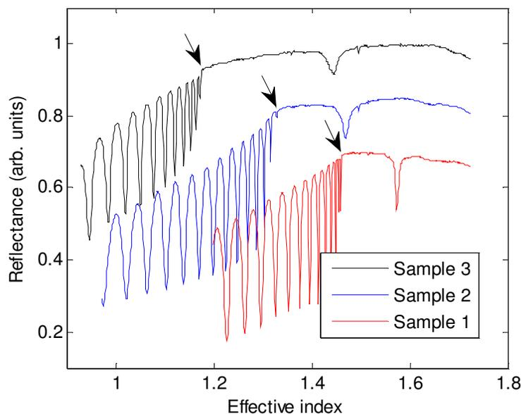
Fig. 1. Dark m-line spectra showing the TE reflectance through a high index prism varying the incidence angle (*i.e.* the effective index). Samples 3 (black), 2 (blue) and 1 (red) with different PS refractive indices are shown. The arrows indicate the PS refractive index in each case, and the isolated peaks show the effective index of the waveguide.
