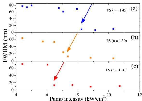
Fig. 4. Full width at half maximum of the emission band at different excitation powers for (a) sample 1, (b) 2, and (c) 3.
